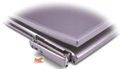
5. Remove the bezel screw and the bezel from the hard drive.
