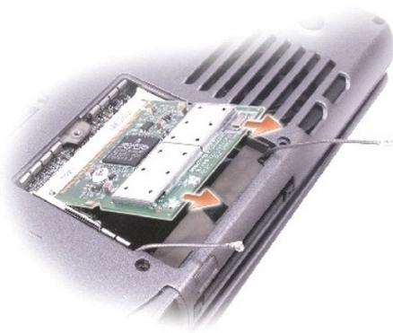
4. If a Mini PCI card is not already installed, go to [step 5](#). If you are replacing a Mini PCI card, remove the existing card:
