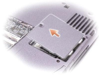
3. Place your finger under the cover at the indentation, and lift and slide the cover open.
