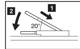
7. Pivot the SO-DIMM downward until it snaps into place.
