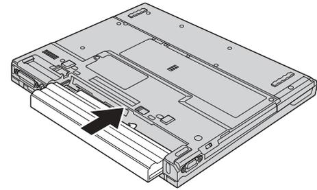
b) Slide the battery latches to the locked position.
