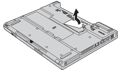
If the SO-DIMM is already in the memory slot, remove it to make room for the new one by pressing out on the latches on both edges of the socket at the same time. Be sure to save it for future use.
